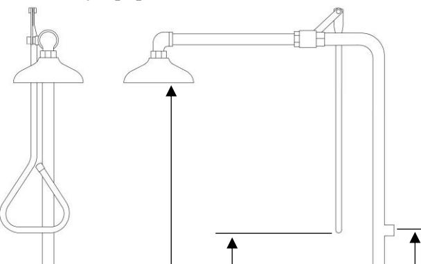
**NOTE:** This unit should be connected to an uninterrupted source of potable water, no less than 25mm with a minimum flowing pressure of 138KPa and a maximum static pressure of 860 KPa.
