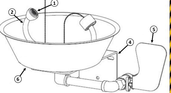
(1) Part No: RPG05-1177 Aerator Screen & Cap Assembly
